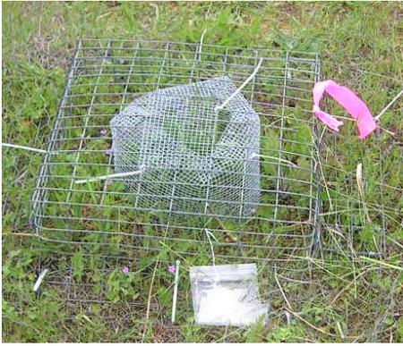
**Figure 4. Enclosure installed inside of enclosure, which was secured to the ground by metal stakes.**
